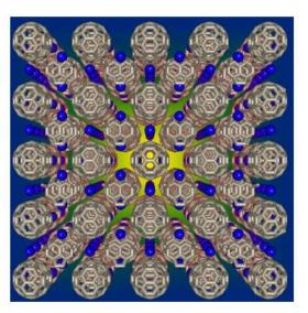
Three-dimensional depiction of the crystal structure of the molecular  $A_3C_{60}$  fulleride superconductors. The fulleren molecules pack in an isotropic cubic-close-packed array in three dimensions. Alkali metal ions (blue spheres) occupy vacant interstitial holes of octahedral and tetrahedral symmetry.
